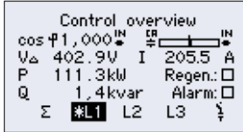
Figure 51 Phase L1 is the control phase
